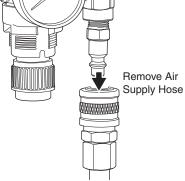
2.3 Remove the elbow connector on nozzle air hose from the nozzle inlet.
