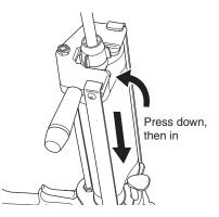
1.4 Attach elbow connector on nozzle air hose firmly onto the nozzle inlet.
